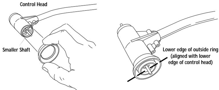
3. After the cement has properly cured (according to the cement's direction), follow the instructions below to attach the wind vane and wind cups to the anemometer.
