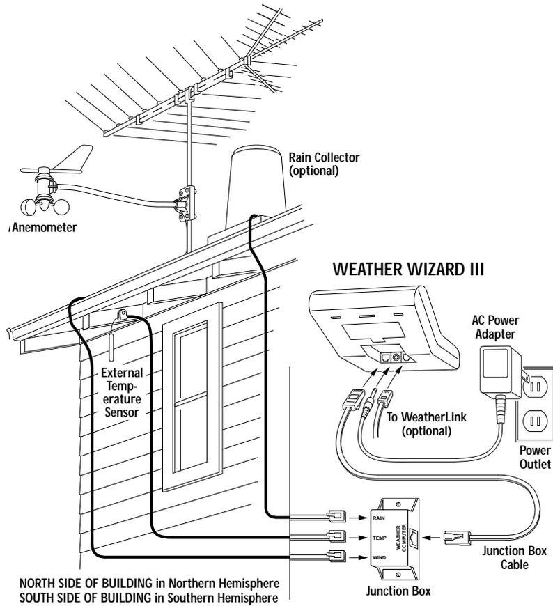
The diagram above shows a typical Weather Wizard III installation. The following pages will give you specific instructions for installing your station. To avoid unnecessary problems, be sure to thoroughly test your system before installing it.
