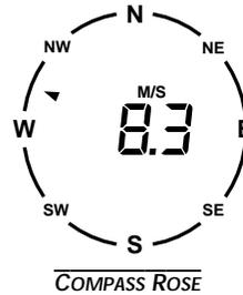
The right side of the display can be set to display Wind Direction in either high (1° increments) or low (10° increments) resolution. Low resolution is probably the most practical setting since even a relatively steady wind has turbulence and rapidly changing speeds. Low resolution gives you a general indication of wind direction—whether the wind is blowing from a northerly or northeasterly direction, for example.
