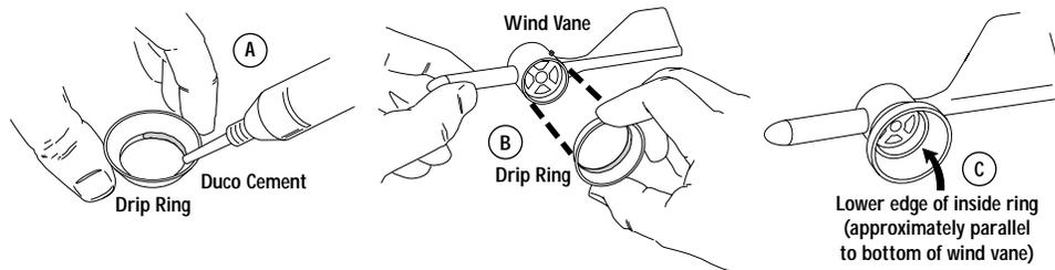
2. Apply adhesive liberally to the inside of the other drip ring and install on the **WIND CUP END OF THE ANEMOMETER CONTROL HEAD** as shown below.
