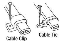
**Note:** Do not use metal staples or a staple gun to secure the cable. Metal staples—especially when installed with a staple gun—have a tendency to cut the cables.
