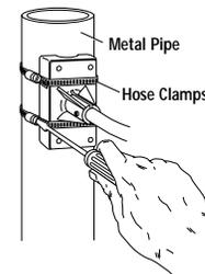
**To Attach the Wind Vane**
