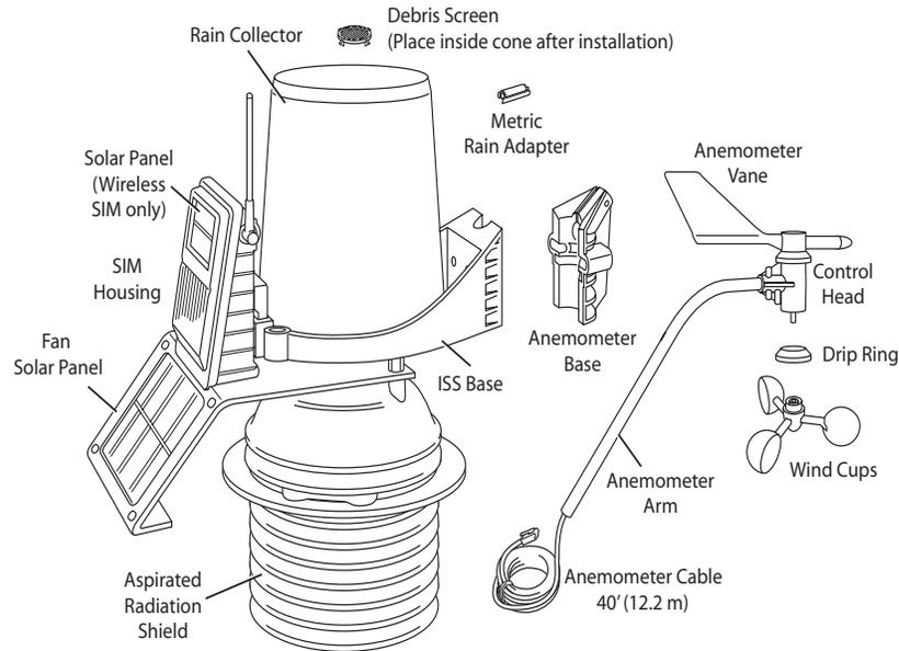
The hardware shown here is provided for assembly and mounting:
