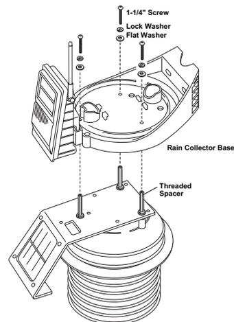
3. Unscrew the three threaded spacers holding the solar bracket and radiation shield together.
