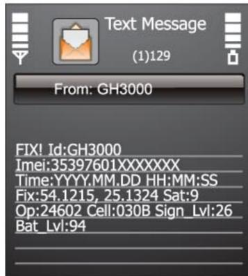
FIX? - GH3000 starts the GPS receiver (if satellites are available), gets location and sends it (in case of reception) to the requesting person. If no current coordinates will be detected device will send the latest coordinates (date/time) from its internal memory.
