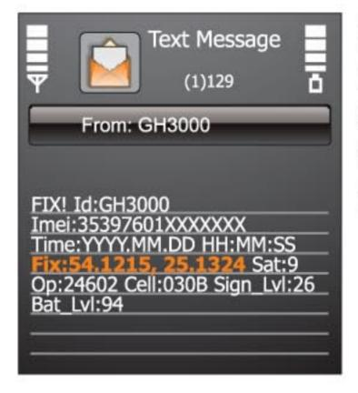
Read received SMS message and find out the word *Fix:* <*numbers*>. These numbers are your device location co-ordinates. If instead numbers is N/A, that means device failed find its location.
