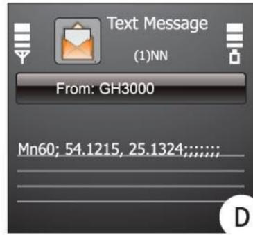
MN? - NAVIGON Mobile Navigator 6 ® (Version 6.3 or higher). After receiving such a SMS GH3000 will send back a SMS to the Mobile Phone and you will be able to see the GH3000 position within the NAVIGON software (on the NAVIGON Map).
