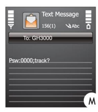
TRACK? - GH3000 will send all collected positions from internal memory to the Server (via GPRS, Server Solution needed).
