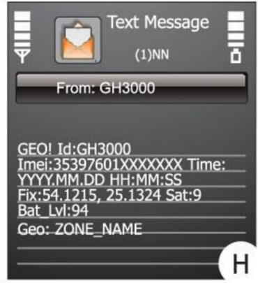
if the device receives request within text Geo? (G) it will find out its location and check if it is in the set zone and send SMS message with the information about them. (H)
