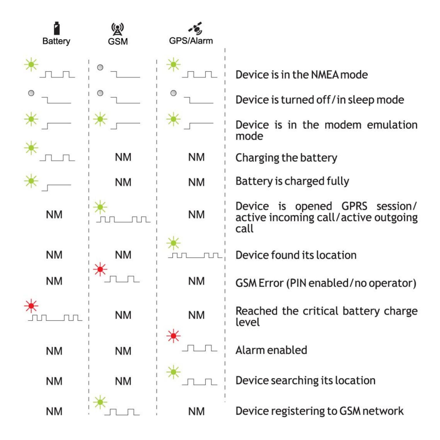
NM - means that it is no matter what LED indicator blinking at the current moment.
