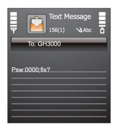
Send SMS request (Fix?) to get location of the device from your mobile phone. Be sure your device is in the open sky, otherwise device will fail to find its location.
